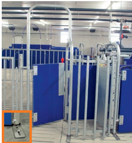
Guiding post with pivoting door Floor fastening made of stainless steel
