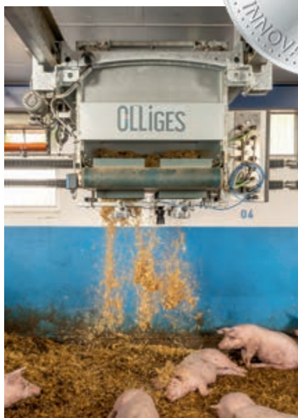
Finishing house: using the OlliGes straw robot significantly reduces the working time required for re-bedding with straw. The robot runs along a rail system to reach any location in the barn
