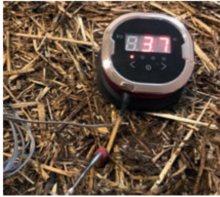
During the batch, a cold composting process occurs at temperatures of approx. 30 to 40 °C
