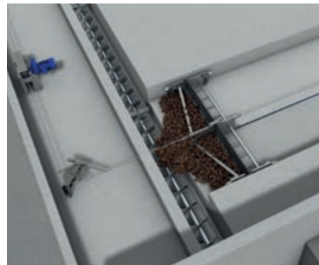
Manure scraper transporting faeces towards cross manure removal
