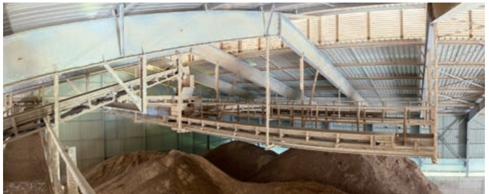
View of a distribution system as conveying system that moves longitudinally with three conveyor belts
