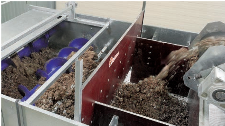
The distributing augers fill the belts evenly
