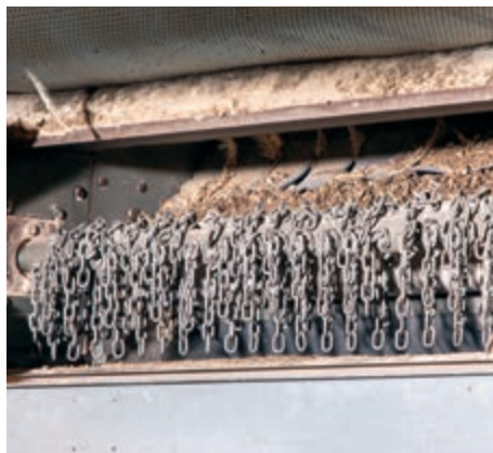
Chopper installed as standard feature with 10 cm long chain links
