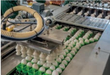
Feed-in system for a continuous egg flow into the farm packer
