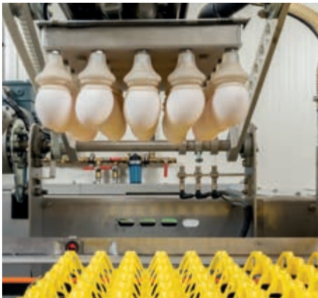
Double-guided transfer arm, horizontal orientation of the suction head during egg placement on the tray and compressed air to ensure very gentle egg handling
