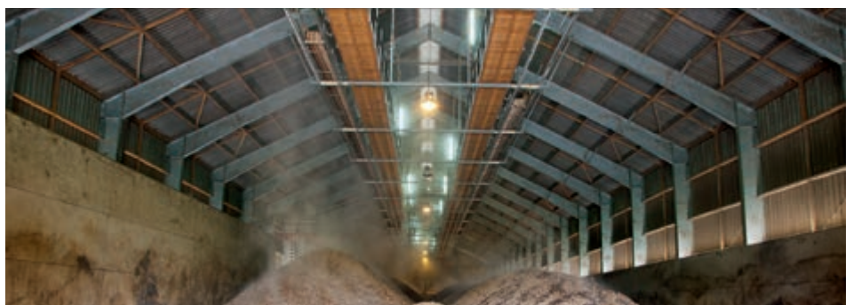
View of a distribution system as conveying system that moves longitudinally with two conveyor belts
