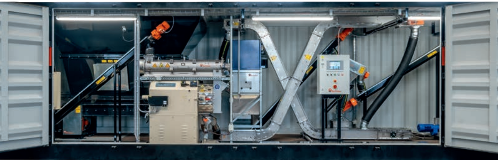
Ready-to-connect delivery of the BD PelletBox 750 in a 40-foot HQ container (12192 mm x 2438 mm x 2896 mm)
