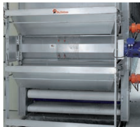
Chopper installed between tiers 3 and 4
