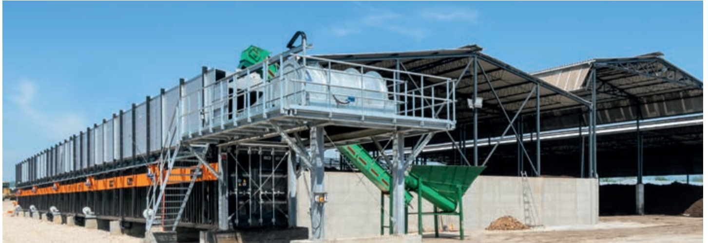
CompoLiner – view of the filling side and the maintenance position of the lane turner
