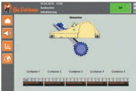
Lane turner with current position of the milling drum
