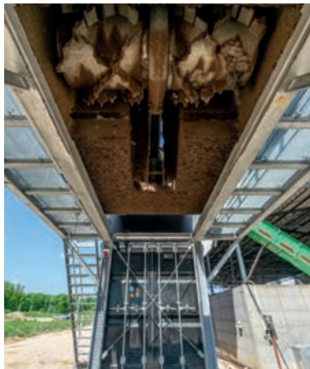
View from below of the lane turner in its parking position – easy maintenance
