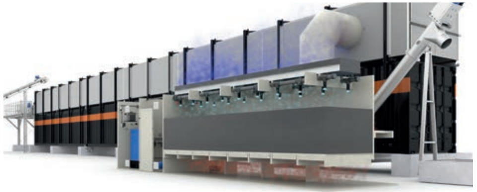
View of the CompoLiner exhaust air cleaner, including technical room and acid store
