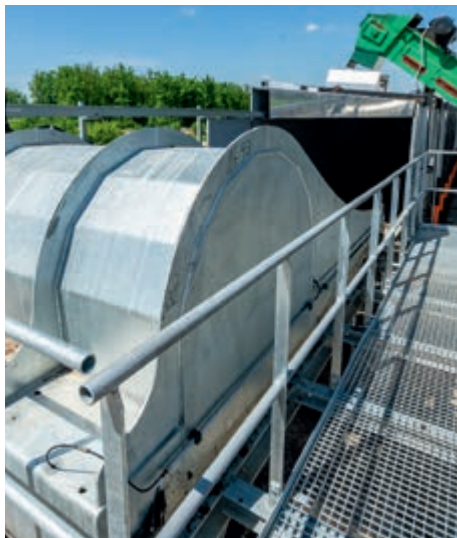
Filling side and parking position of the lane turner
