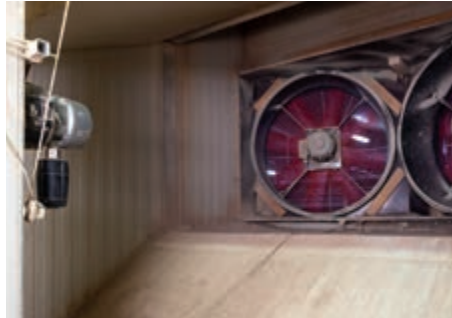
Measuring the NH 3 concentration in the exhaust air (with a separate display for testing purposes)
