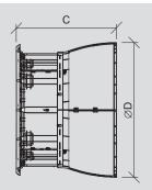
The fan must be equipped with a wire mesh guard in front of the shutter where it is installed at a height of less than 2.70 m and accessible by people.
